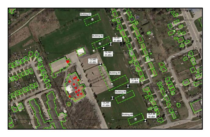
**Building #1** • Warning Clause Type C for the East and South façades. • Requirement for Air Conditioning for the entire building. These have been summarized in Attachment B under Table B1.
